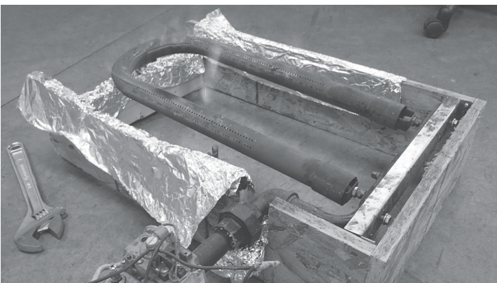
Figure 4. Horseshoe Shaped Gas Burner
