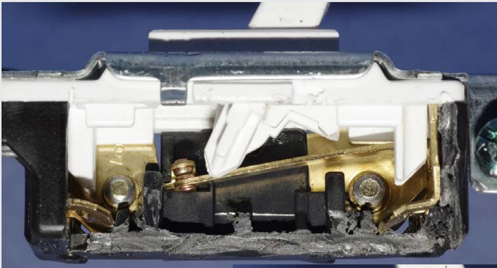
Typical Single Pole Residential Switch in the ON Position
